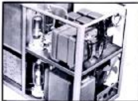
Interior view showing conservatively rated power equipment, heavy-duty modulator.
